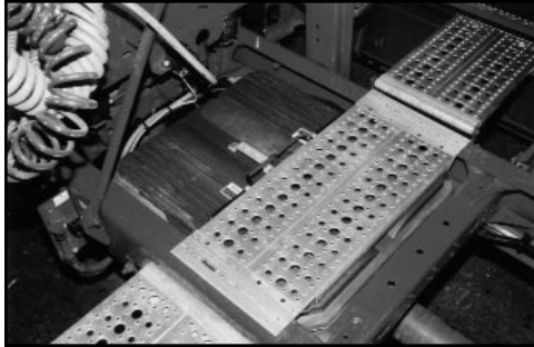
Columbia: battery box behind cab
