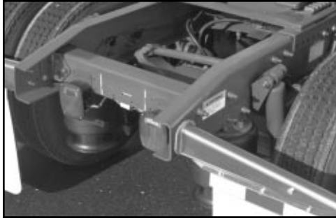
Columbia: AirLiner suspension
