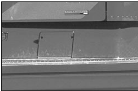
Columbia: fuel tank fill, door closed
