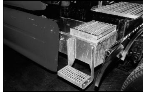
387: battery box behind cab
