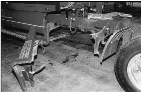
Columbia: rear fairing removed
