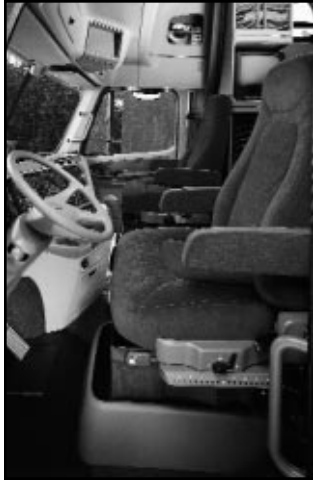
Columbia: driver entry with "B" pillar grab handle
